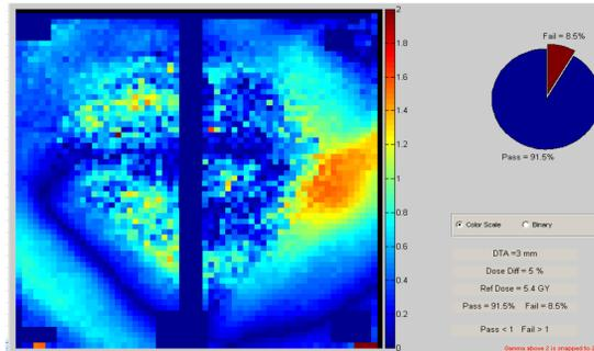
**Figure 3.** Coronal film gamma analysis for Trial 1 of the passive scattering plan
