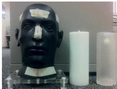
**Figure 2.** Head phantom with dosimetry insert (L) and imaging insert (R)
