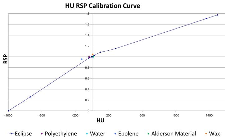
**Figure 1.** The HU-RSP calibration curve for the Eclipse treatment planning system, with phantom materials plotted
